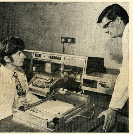
In the biochemistry department at Queen's University, David Jamison (right) who designed and developed the graph reader, discusses an application with Arthur Davies, a post-graduate research student, who is selecting the points along the graph.
