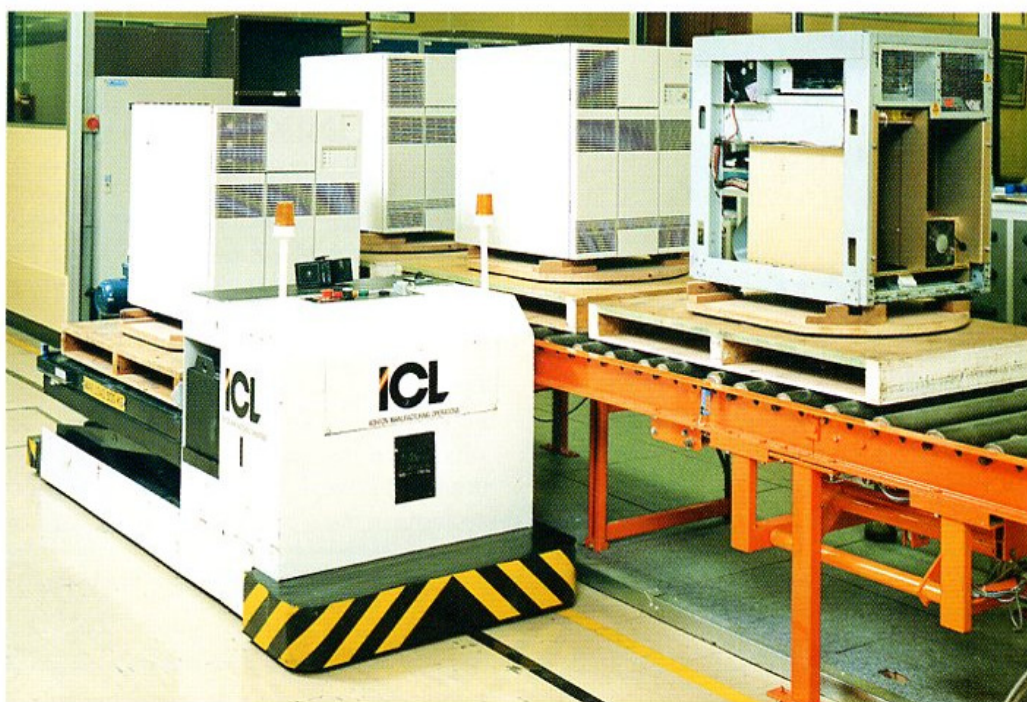
The DRS 6000 servers are manufactured in ICL's plant at Ashton-under-Lyne which was chosen as one of the 'Five Best British' factories in 1989. In this picture, an automated guided vehicle is lifting a completed DRS 6000 server from the end of the computer-controlled assembly line.
